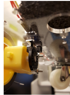
(b) Bottom view of encoders
